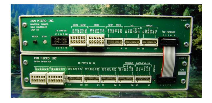
Will detect and generate alarms from IN32B modules, build and dispatch alarm messages to displays, pagers, wireless phones. Will also store call statistics for Jsm Report reporting software.
